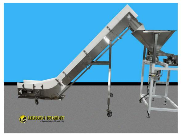
For this application, an infeed conveyor was provided that received the roasted peanuts directly from the customer's roaster.
