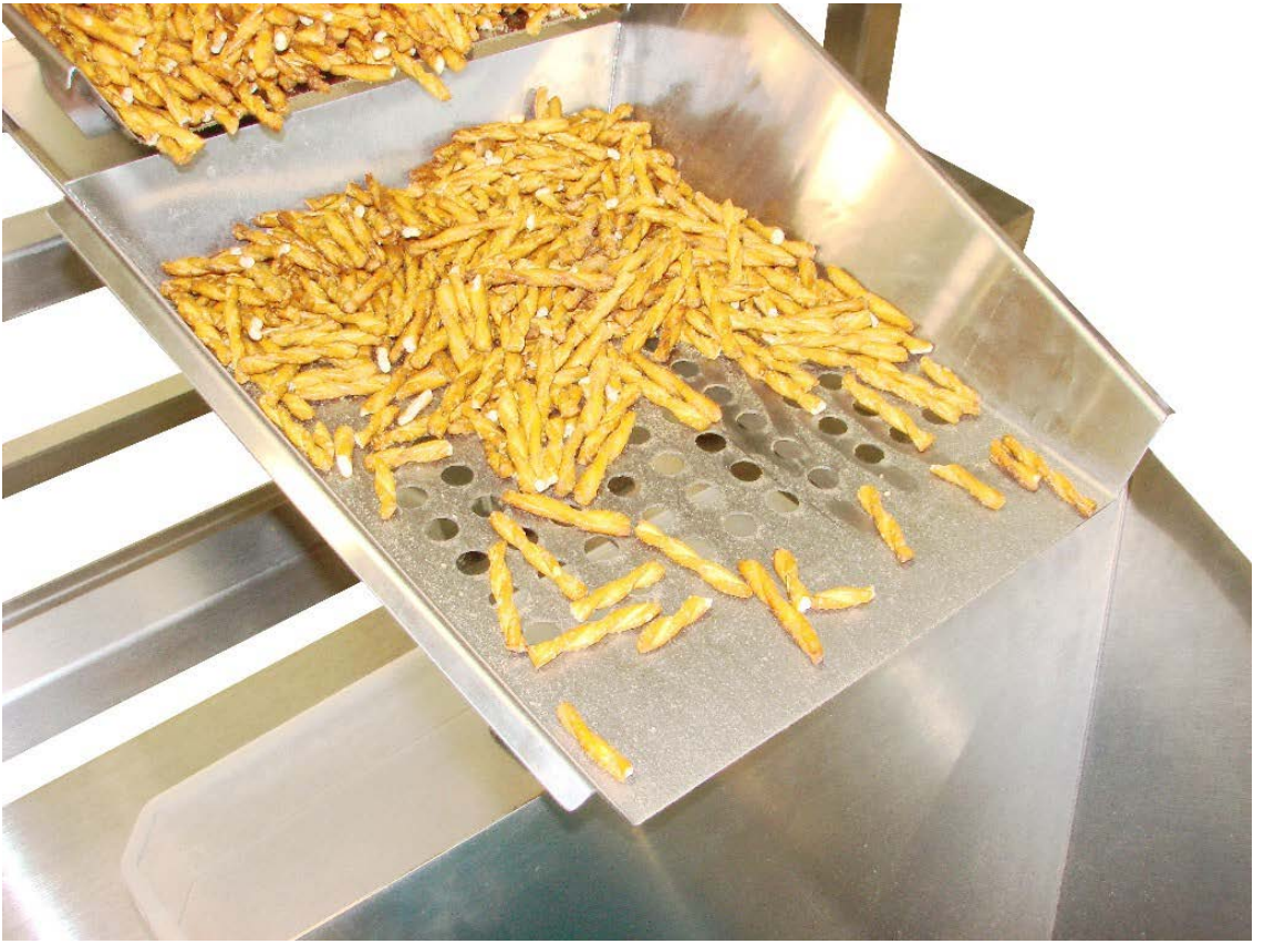
Shown Above: Perforated tray allowing small fines to be discarded before going to the scale and packaged.
