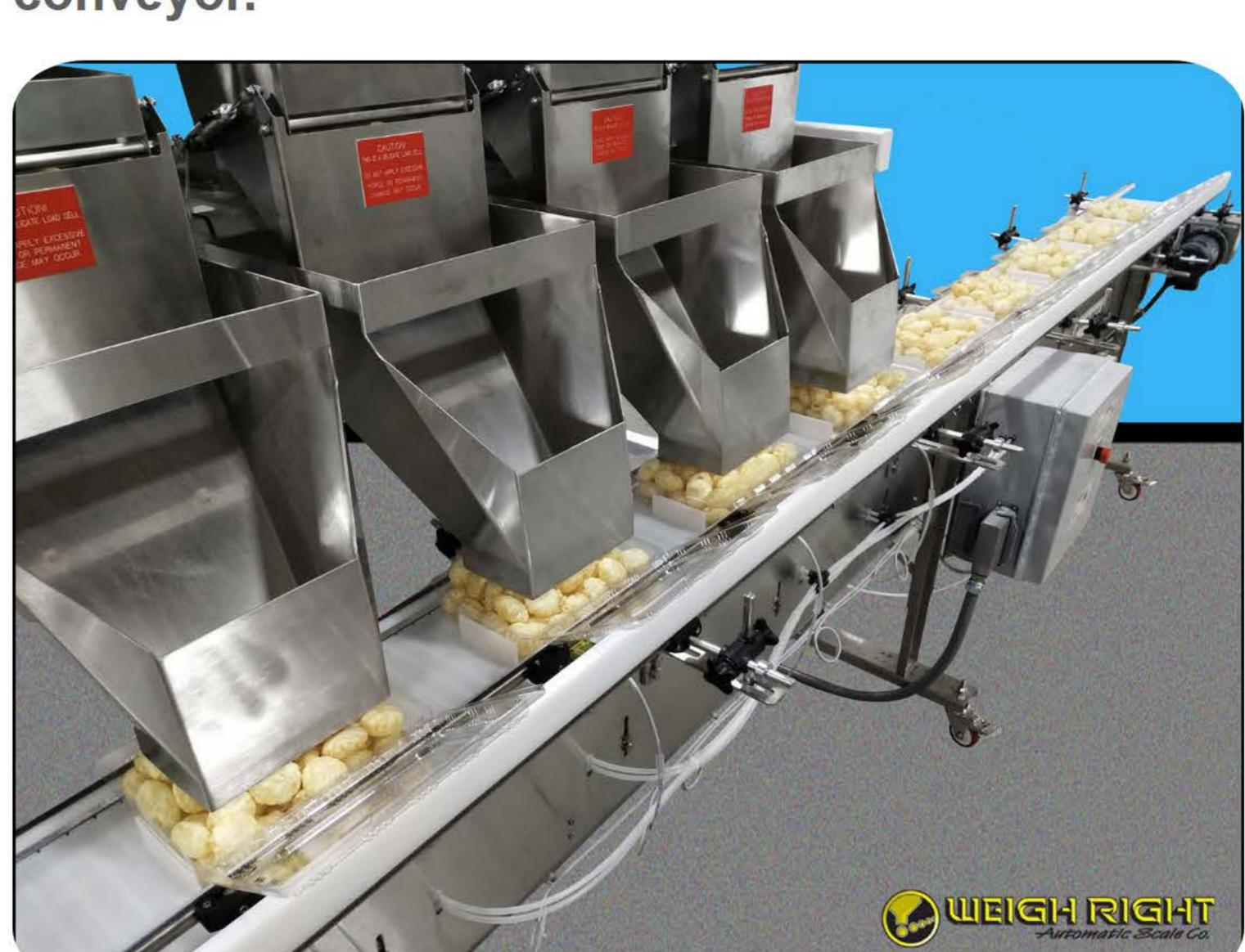
Product gently slides out of the weigh buckets and into the clamshell trays. Conveyor features underbelt vibrators to settle product.
