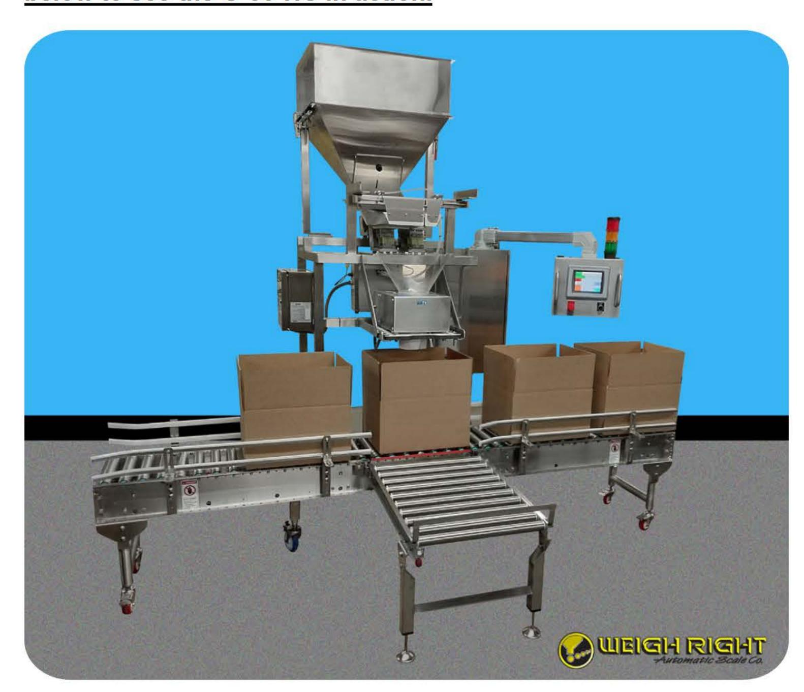
G-50-HC Scale shown optional Metal Detector Support (MD supplied by others), Reject Conveyor, Pendant Arm, Light Tower and Allen Bradley Controls
