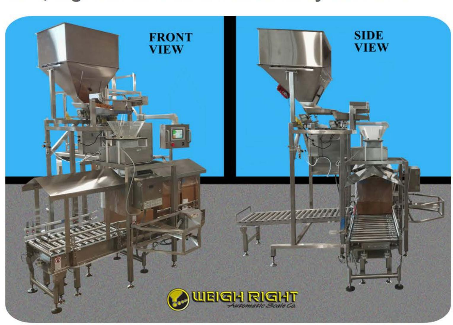
G-50-HC Customized for our customer to include Product Dust Shield, Reverse Carton Reject if metal detected, and Supply Hopper Extension
