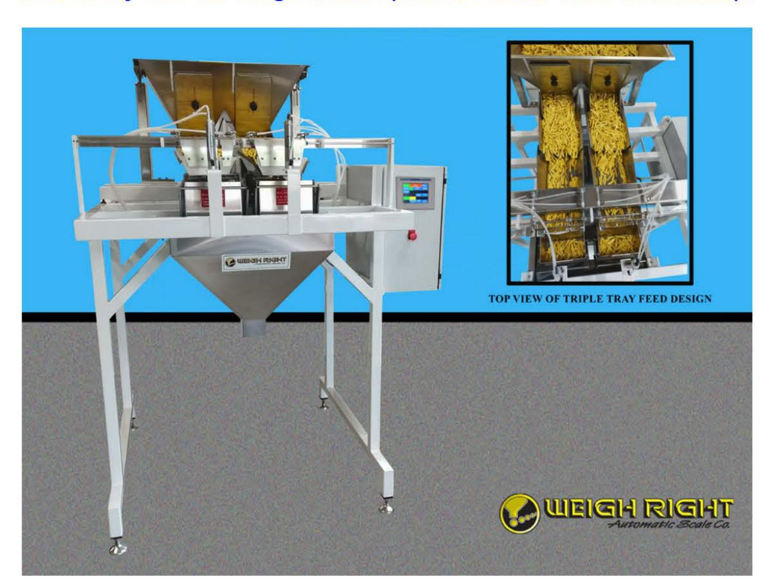
Shown Above: PMB-2 Scale with custom frame to mount over a bagger. 1 to 6 lane scales are offered depending on speed requirement or if blending products.
