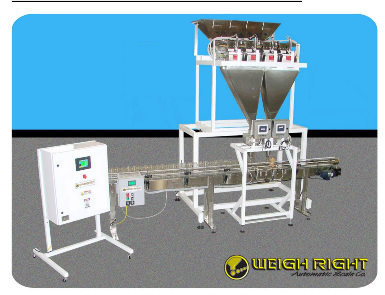
PMB-4 Scale with dual discharge hoppers feeding through metal detectors into jars indexed by our HC-10 conveyor (metal detectors provided by others).
