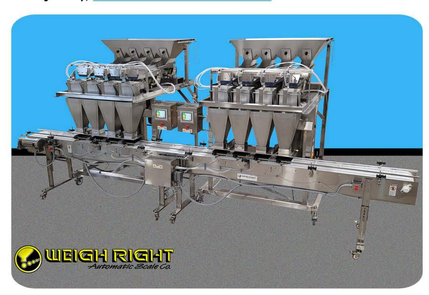
PMB-4 USDA Scales shown with HC-20 tray indexing conveyor.
