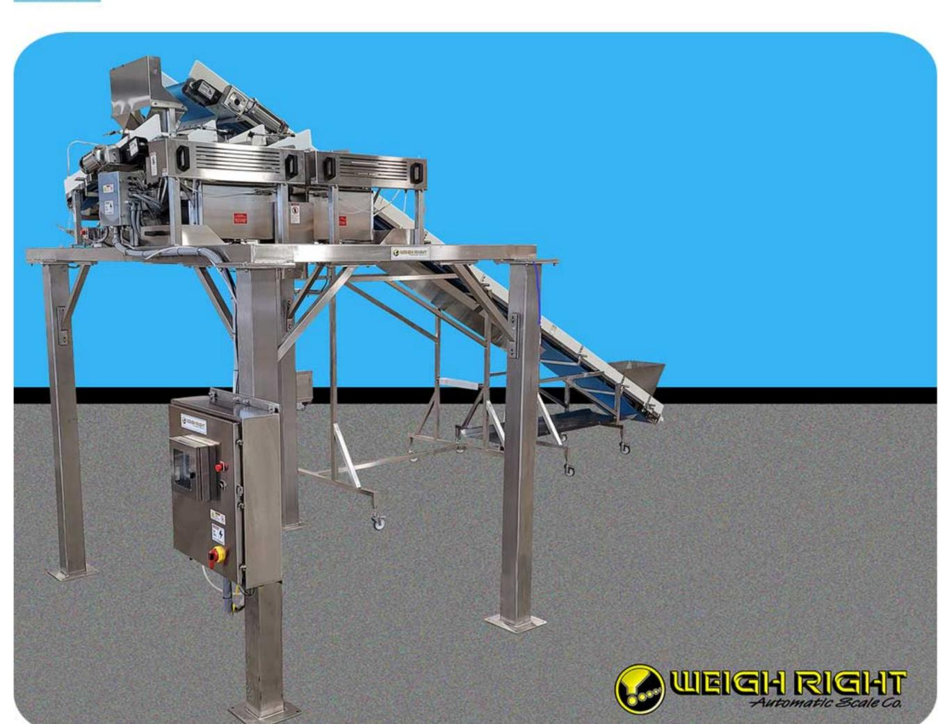
BDC-2 shown with stainless frame to mount over vertical bagger (made by others) and infeed conveyor.
