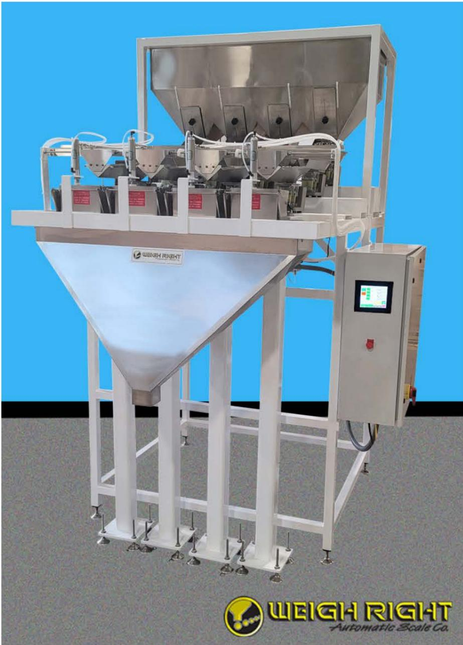
Shown Above: PMB-4 Scale with isolated load cell columns.
