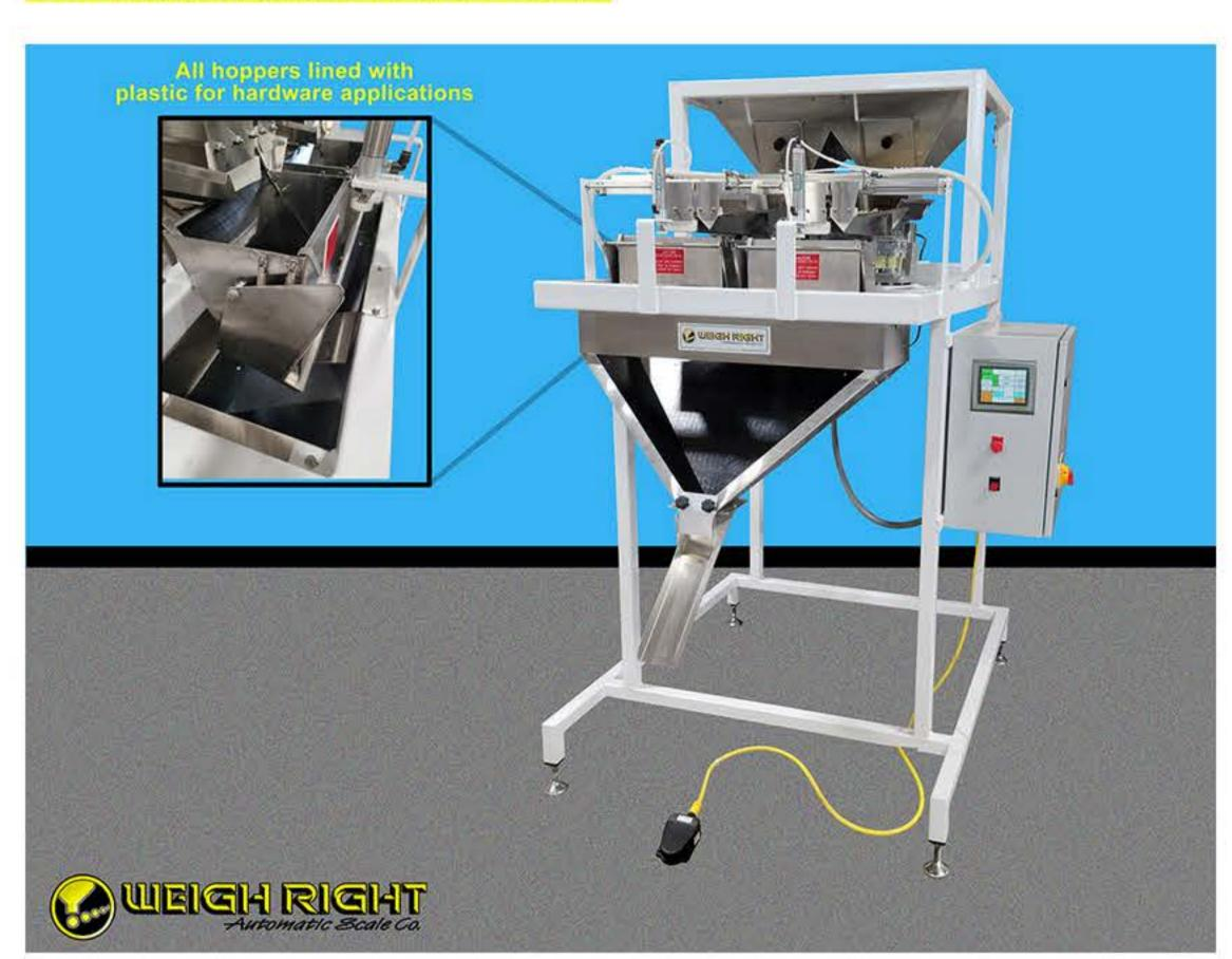
Shown Above: PMB-2 Scale designed for packaging hardware into bags in a semi-automatic operation requiring and operator to hand-place the bag for filling.
