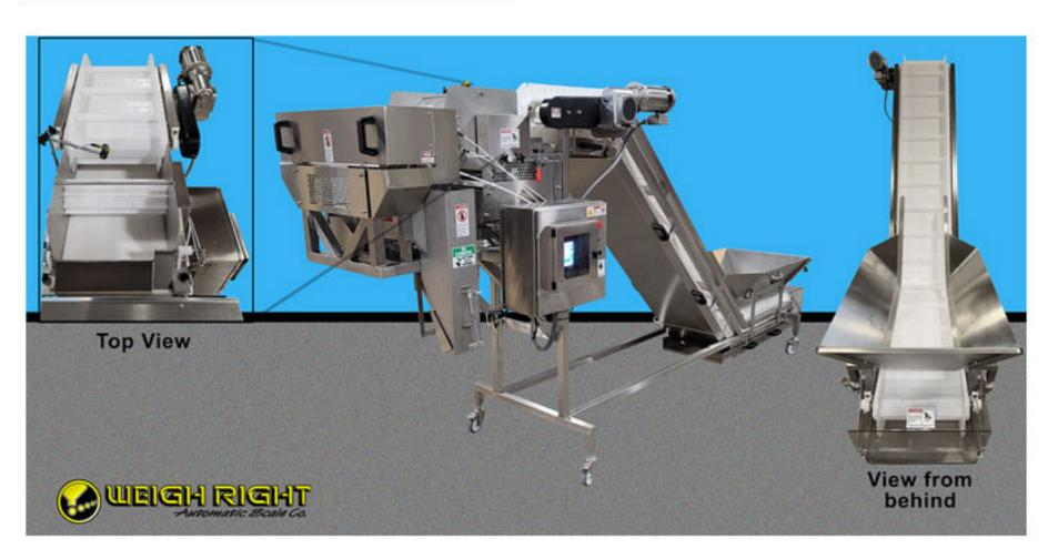
Shown Above: FCS-1 with loading hopper and top view of the bulk / dribble belt and infeed conveyor.
