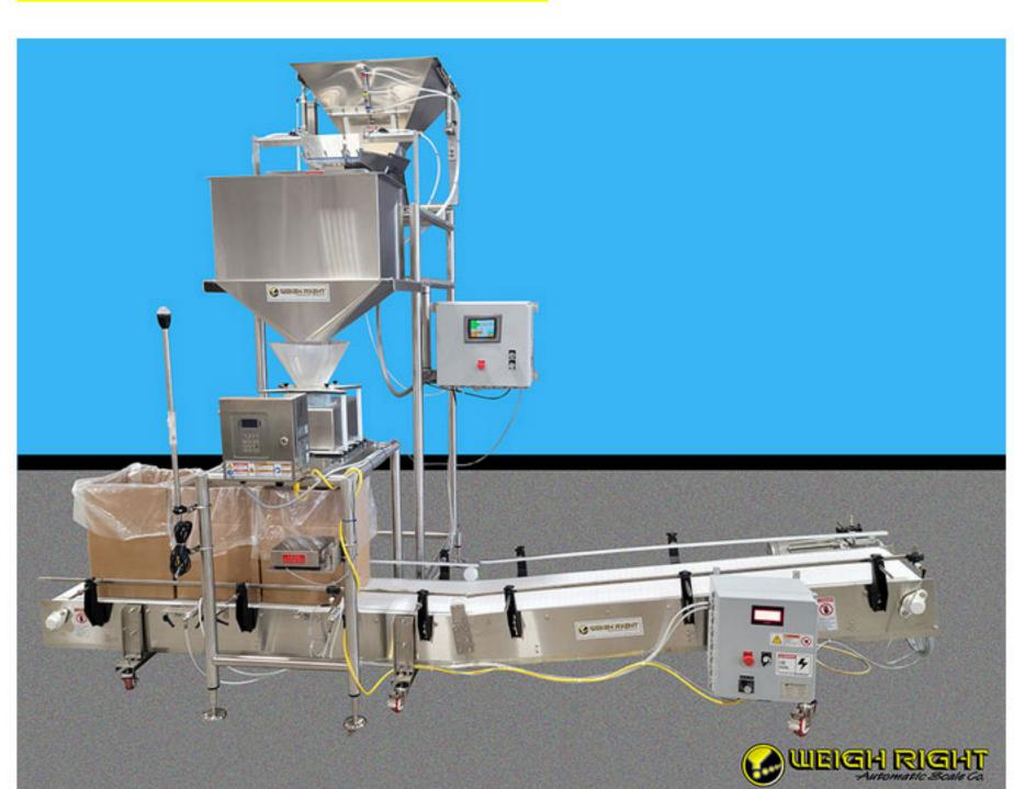
Shown Above: PMB-3601 bulk filling scale with angled case conveyor and flow-thru metal detector (provided by others, mounted by Weigh Right).
