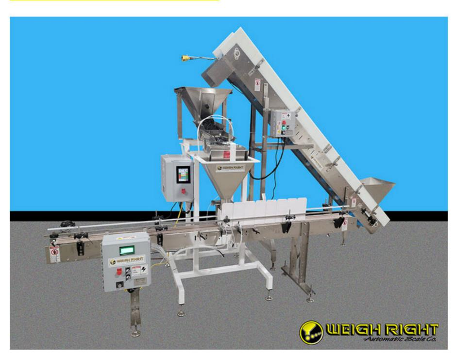
**Shown Above:** The iQ-1E scale with our IC-45 infeed conveyor and HC-10 indexing conveyor.
